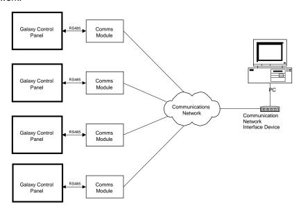
This type of configuration is designed for organisations requiring servicing and controlling multiple remote sites, enabling the information contained on each site to be copied, stored and overwritten using the PC. The stored information can also be modified using the off-line programming facility, enabling Galaxy sites to be programmed and stored on the PC in advance of commissioning the control panel.
