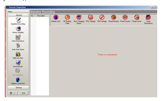
The window is split into two parts: the General menu baselines down the left-hand side and the data associated with each baseline on the right-hand side.
